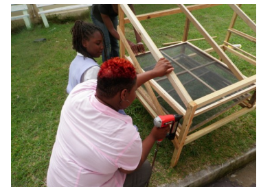
5. Nail in runners, join a 2"x1" with a 1"x1"
